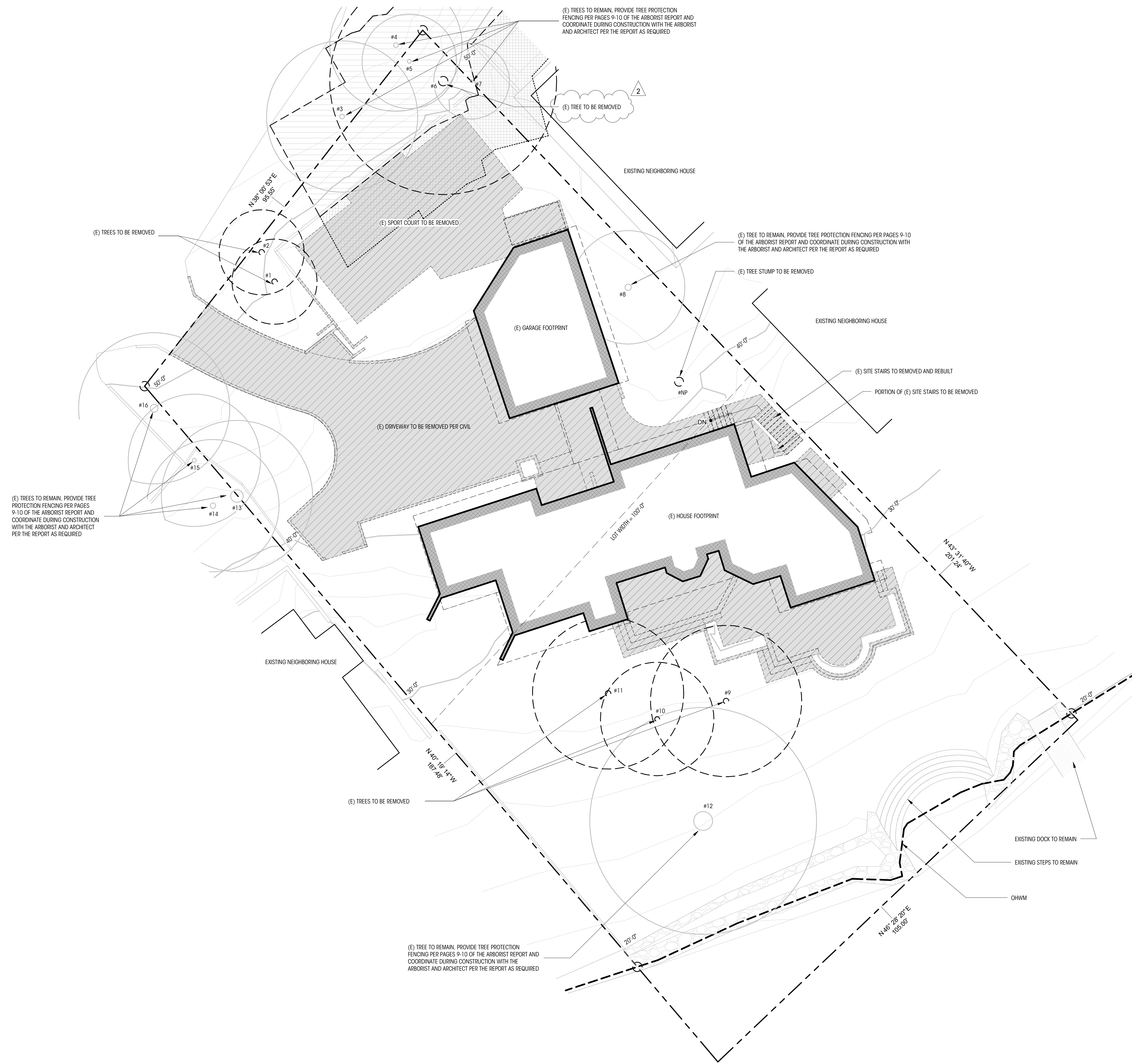
1 SITE DEMOLITION PLAN 1" = 10'-0"
